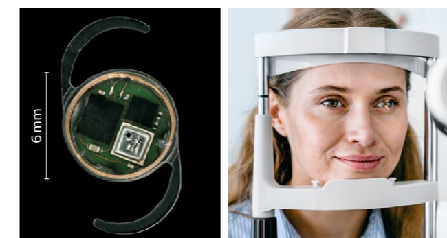
Development of a wireless implantable intraocular pressure sensor (WIPS) for glaucoma patients. Through the transmitted data, the medical team can evaluate the effectiveness of current treatments for patients in real time.
