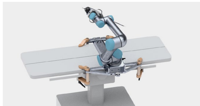
Robotic arm system for tool development – The development of surgical instruments requires extensive testing and evaluation. To help our client evaluate various designs and accelerate the product development cycle, we developed and built a “surrogate” robotic arm system, enabling quantitative evaluation of the performance of new instruments in a pre-clinical environment, with surgeons controlling the arm and trying out the new designs.
